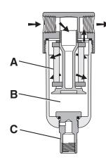
The contaminated air enters the element interior and is forced through a thick membrane (A) of "borosilicate" glass fibers coated with epoxy. Flow then passes through the element, and at this stage 99.97% of the sub micronic particles have been removed from the air stream. The tiny droplets coalesce together and are collected from the filter element by the outer drain layer.
