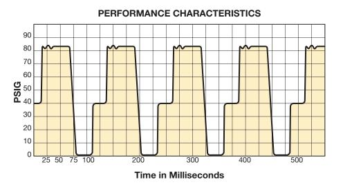
Actual test results show rapid response on a robot welding operation at a major U.S. automotive manufacturer.
