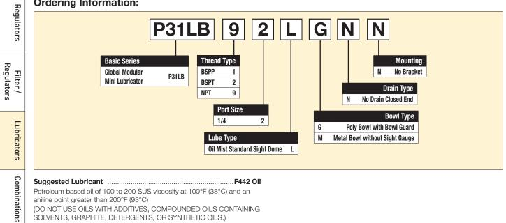
Petroleum based oil of 100 to 200 SUS viscosity at 100°F (38°C) and an aniline point greater than 200°F (93°C)
