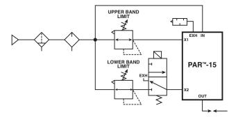
Note: For valves with normally open solenoids, reverse the X1 and X2 connections.
