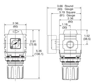
Inches (mm) NOTE: 1.90 in. (48mm) hole required for panel nut mounting.
