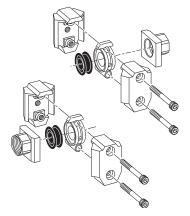
Port block connectors allow you to make threaded port connections to modular units and are available in various port sizes to match your system requirements.
