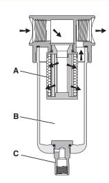
The contaminated air enters the element interior and is forced through a thick membrane **(A)** of "borosilicate" glass fibers coated with epoxy. Flow then passes through the element, and at this stage 99.9997% of the sub micronic particles have been removed from the air stream. The tiny droplets coalesce together and are collected from the filter element by the outer drain layer.
