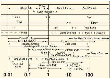
To assist in understanding the parameters of filtration, refer to this pollution size comparison chart. Look at the size of a major contaminant, oil aerosol! It is in the region of 0.01 - 0.8 micron. Tobacco smoke is also a liquid aerosol in a similar size band 0.01 -1.2 micron. Observe the smoke test yourself, appreciate the size of the problem! The smallest particle the human eye can see is in the order of 40 microns.
