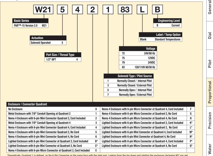
Theoretically, Quadrant 1 is defined as the 6-Pin Connector on the same face with the inlet port. Looking from the top down and rotating the enclosure clockwise 90° you get Quadrant 2 or 270° for Quadrant 4.
