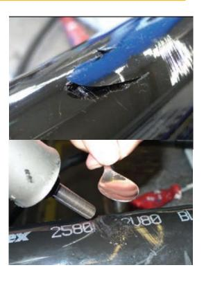
Appendix 3: Procedure for a repair of a local damage in the outer cover
