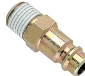
88103304 IBN/IBS Series nipple, 3/8" male thread, 8 mm bore (ISO6150B / MIL-C4109)
